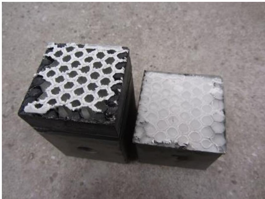
Photo No. 6 Aluminum Rear Face / Honeycomb Core Bond Failure Mode Detail
