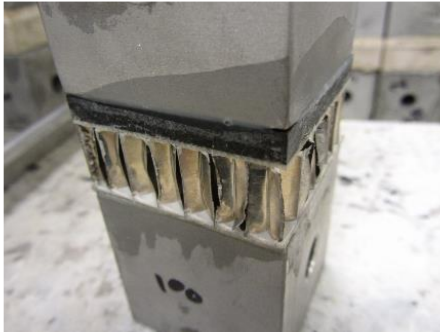
Photo No. 7 Representative High-Exposure Cycling (100 Cycles Completed) Unsealed Edge Specimen Showing Deformation of Honeycomb Core from Interior Water Freezing/Expansion
