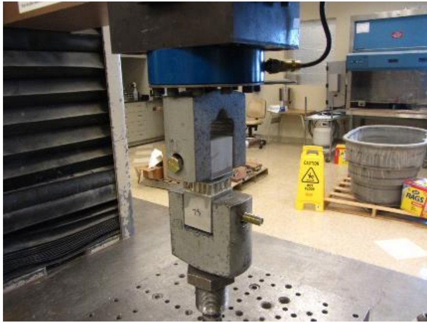
Photo No. 3 ASTM C297 Flatwise Tensile Bond Strength Test Apparatus – Unsealed Specimen
