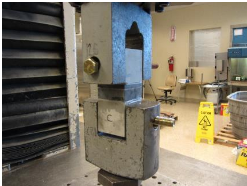
Photo No. 4 ASTM C297 Flatwise Tensile Bond Evaluation Loading Detail – Sealed Specimen
