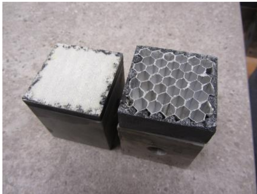
Photo No. 10 Representative Light Adhesive Application Bond Layer Detail – Sealed Specimen
